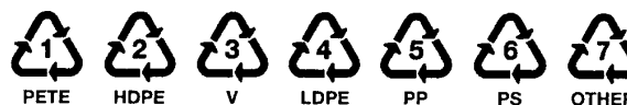
Figure C. Recycling symbols indicate types of plastics each resin has its own properties such as specific melting temperatures and processing qualities. The four most common nursery plastics are marked with an asterisk (Table 2):
