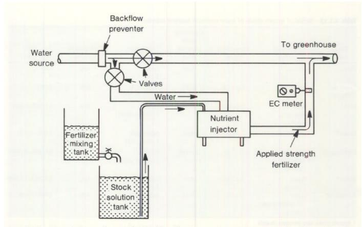
Figure 4.1.17—Schematic diagram of a typical liquid fertilizer injection system for a container nursery (adapted from Nelson 1978).
