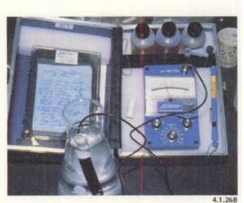
Figure 4.1.26—Every container nursery should have certain irrigation and fertilization monitoring equipment. Electrical conductivity meters (A) can be used to measure soluble salts, and a pH meter (B) can be used to monitor the pH of irrigation water and applied fertilizer solutions.
