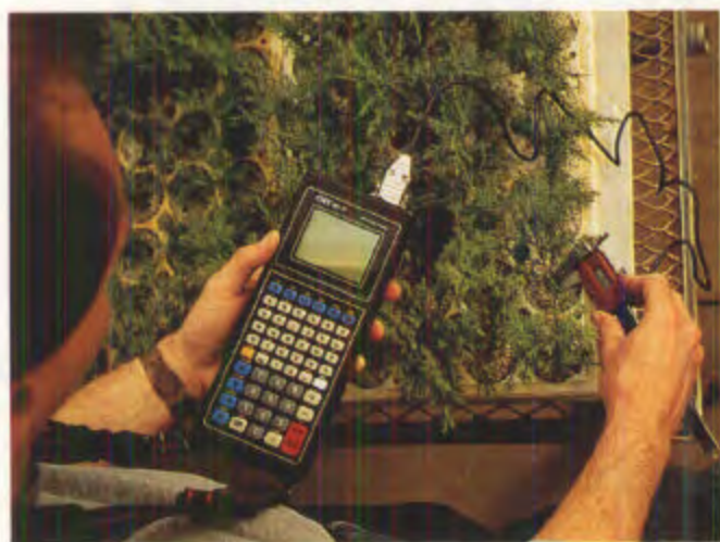
Figure 1.5.4 —Regular monitoring of seedling growth (A) provides information on the effectiveness of cultural practices, and also is a good time to check for pests. New digital calipers can be read with portable data recorders, making seedling growth monitoring quick and accurate (B).
