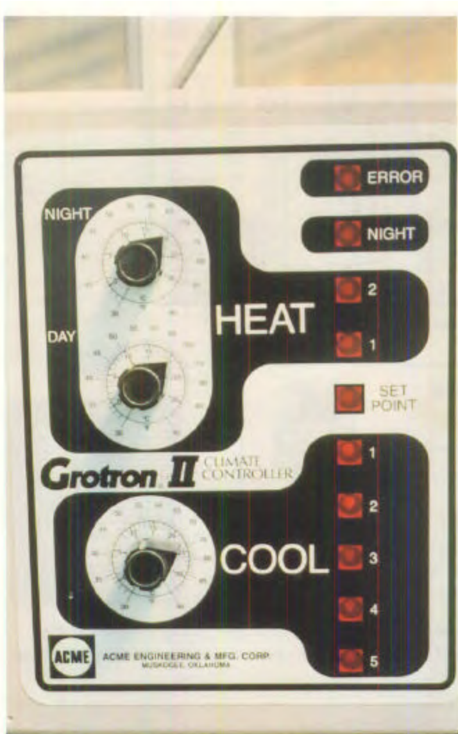
Figure 1.4.8 —Climate controllers regulate heating and cooling in a series of stages around the desired set point temperature.
