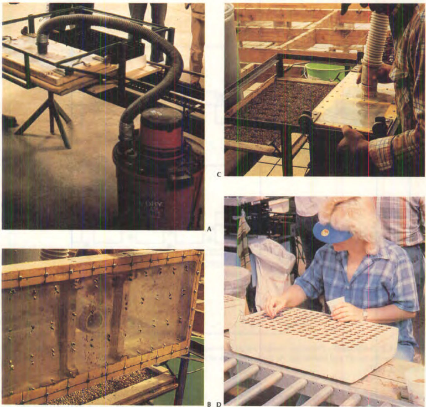
Figure 1.4.26 —Vacuum plate seeders (A) pick up seeds and hold them on the hollow head in the same grid pattern as the cells in the container. The number of holes determines the sowing density (B). When the vacuum is released, the entire container is sown at once (C). Both shutterboxes and vacuum plate seeders require monitoring and often extra seeds need to be sown in blank containers (D).
