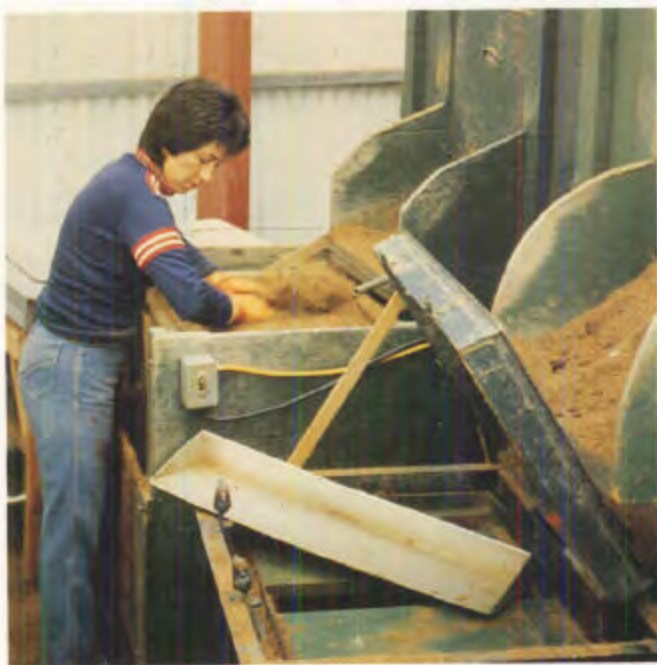
Figure 1.4.24 —Homemade container filling equipment uses a vibrating or shaking motion to eliminate air pockets (A); more sophisticated commercial models offer recycling of media and other features (B). Filled containers are dibbled to compact the media and produce a space for the seed, either by hand (C) or as part of the mechanical sowing line (D).
