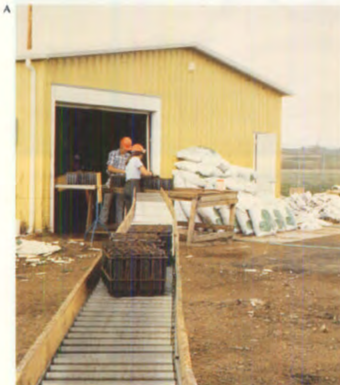
Figure 1.4.17 —Several types of conveyors are available for use throughout the nursery system. Roller conveyors (A) are unpowered but belt conveyors (B) and chain conveyors (C) use electrical motors to transport containers or materials.
