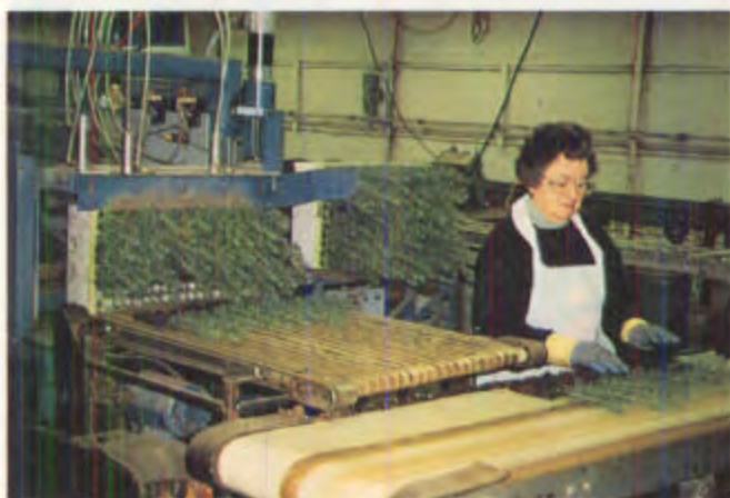
Figure 1.4.32 —New equipment is being developed to make seedlings easier to pull from the container. Mechanical thumpers (A) loosen the seedlings with a jarring motion and then the seedlings can be pushed from the container onto the grading belt with an extractor (B). Graders count and bundle the seedlings into plastic bags (C) or bind the root plugs together with plastic wrap (D).
