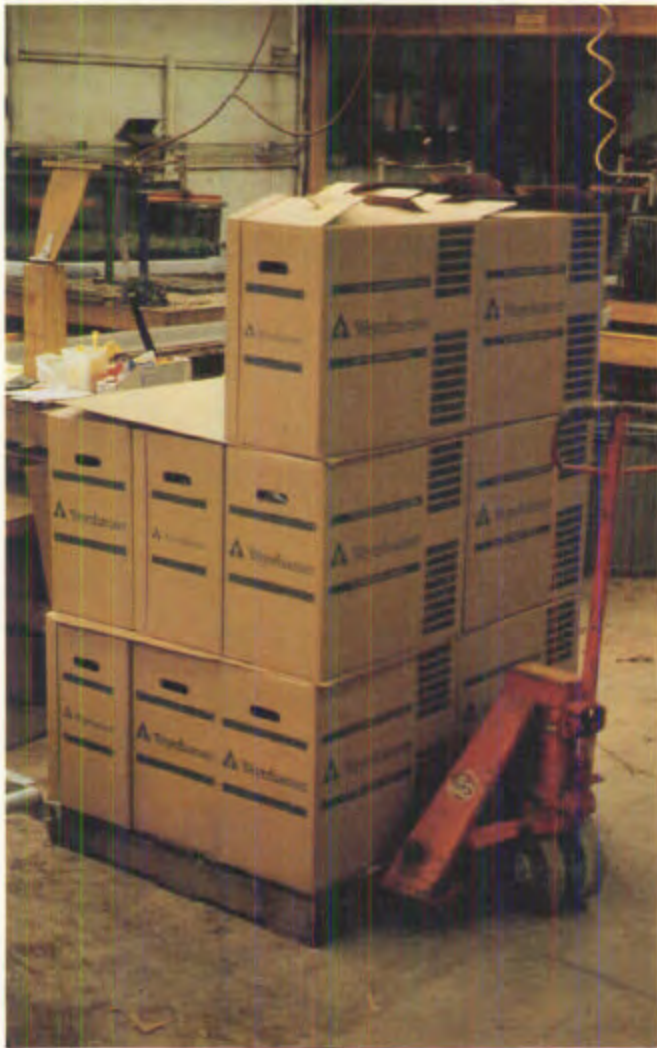
Figure 1.4.18 —Containers and supplies are handled by pallet jacks (A), fork lifts (B), or carts (C), which must be powered by propane or electricity in closed areas for safety reasons. Fuel-powered tractors and trailers can be specially modified to transport seedlings in open growing areas (D).
