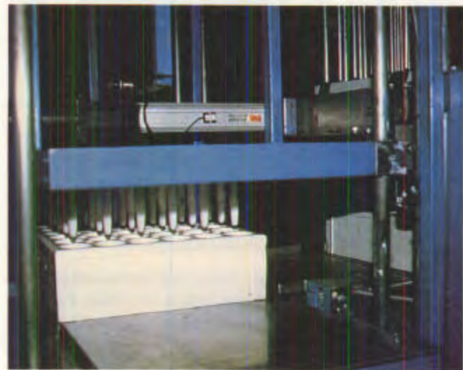
Figure 1.4.29 —Transplanting young seedlings from miniature containers into larger containers is a new technology that shows promise. The large containers are predibbled (A) and then the miniature seedlings are transplanted downward into the cavity (B). (Courtesy of Beaver Plastics Ltd., Edmonton, AB.)
