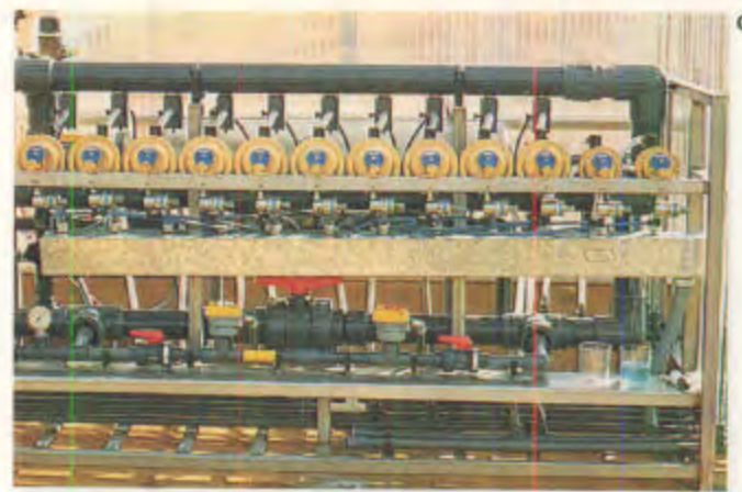
Figure 1.4.7 —Injection of fertilizer solutions into the irrigation system (fertigation) is an efficient way to supply mineral nutrients (A). Granular fertilizers, like these Osmocote® pellets, can be incorporated into the growing medium (B). Computerized fertigation systems are now being used to precisely control mineral nutrient injection (C). (C, courtesy of E. Labbate, Climate Control Systems, Leamington, ON.)
