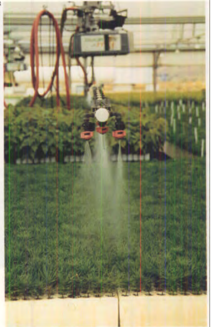
Figure 1.4.6 —Fixed irrigation systems use sprinkler nozzles that throw a circular pattern (A); movable boom systems distribute an even curtain of water over sections of the growing area (B). Weighing sample containers is a fast and easy way to monitor water use by seedlings (C).
