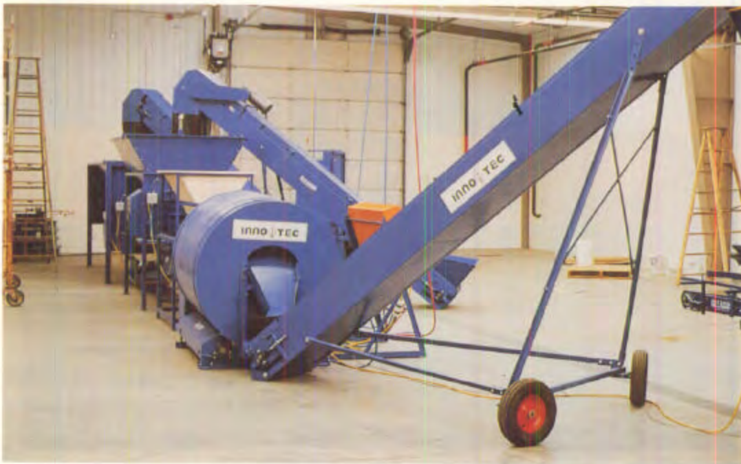
Figure 1.4.22 —Small quantities of growing medium can be mixed by hand or in cement mixers (A), but larger nurseries use batch mixers to keep the filling and sowing line supplied with medium (B). Continuous mixing equipment is designed to ensure even mixing and distribute incorporated materials without breaking down the physical structure of the components (C). (C, courtesy of J. Reid, Inno-Tec, Thunder Bay, ON.)
