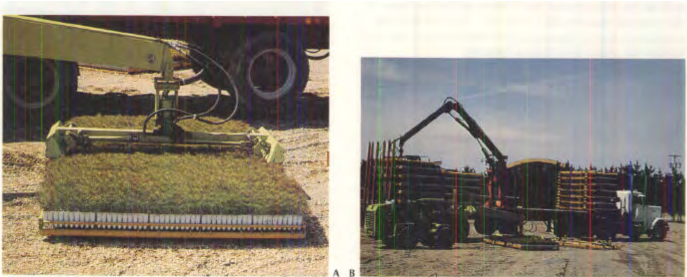
Figure 1.4.16 —Container handling systems move seedlings from the propagation area, to the hardening area (A) and then to the outplanting sites (B) and some are quite sophisticated.
