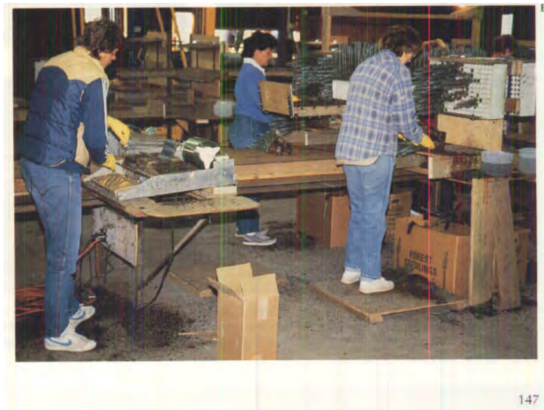
Figure 1.4.31 —Seedlings that are shipped to the outplanting site in their containers are boxed or stored on racks (A), so that they are protected during transport. Many nurseries process their seedlings in a packing line where the seedlings are pulled from the container, then graded, bundled, and boxed for storage and shipping (B).
