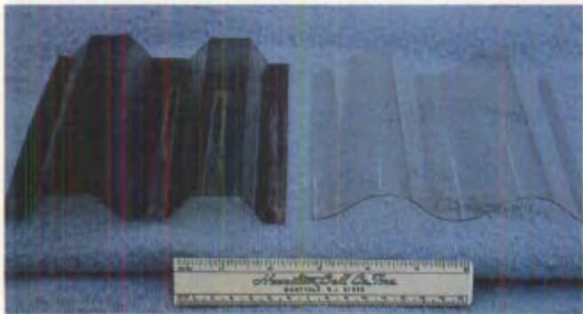
Figure 1.3.16 —One of the first types of rigid plastic panels was fiberglass-reinforced polyester but it tended to yellow with age (A). Several new structured plastic panels are now available in single-layer corrugated (B) or double-layer flat sheets (C), which are flexible enough to cover quonset structures (D). (Samples in B&C courtesy of Co-Ex Corporation, Rocky Hill, CT.)
