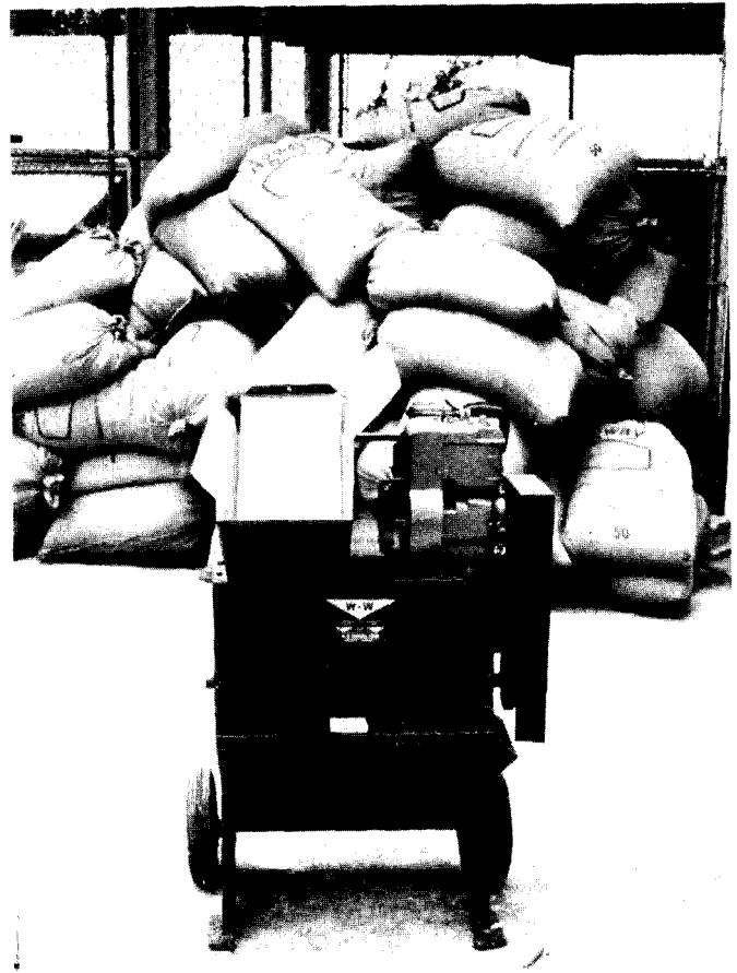
Figure 15-7.-A small, very mobile, gas-powered compost shredder capable of processing 7 \text{ m}^3 per hour of rice hulls, sugarcane waste, straw, and other materials.
