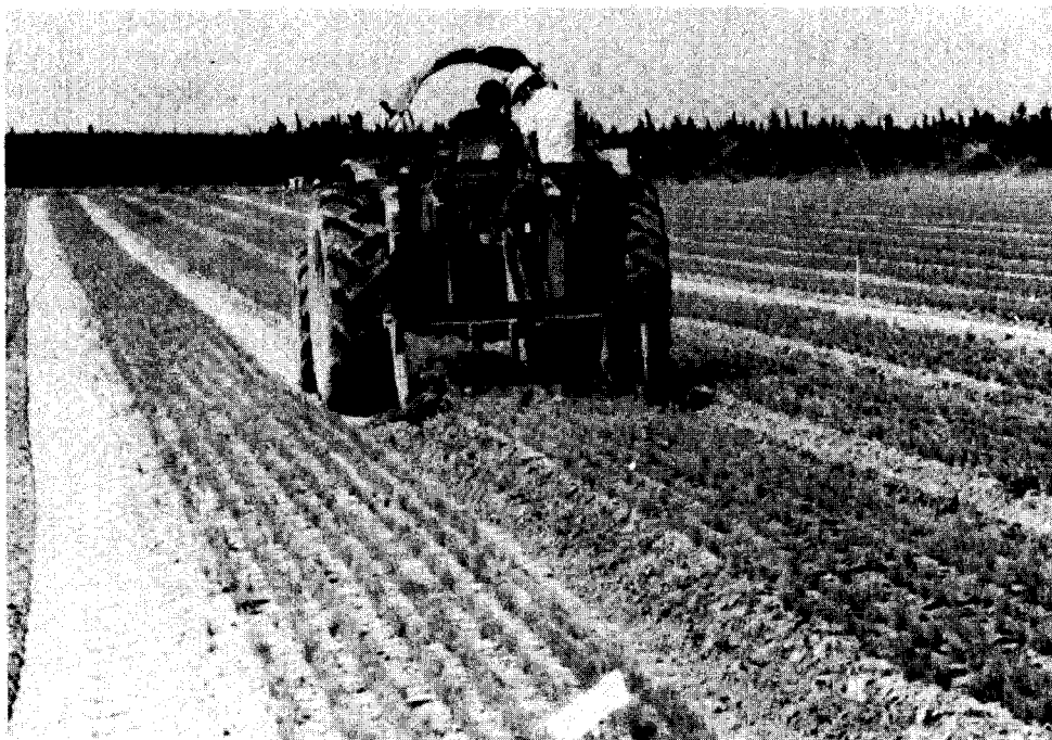
Figure 16-1.-A hydraulic tractor-mounted blade being used for undercutting pine seedlings on raised or mounded seedbeds.
