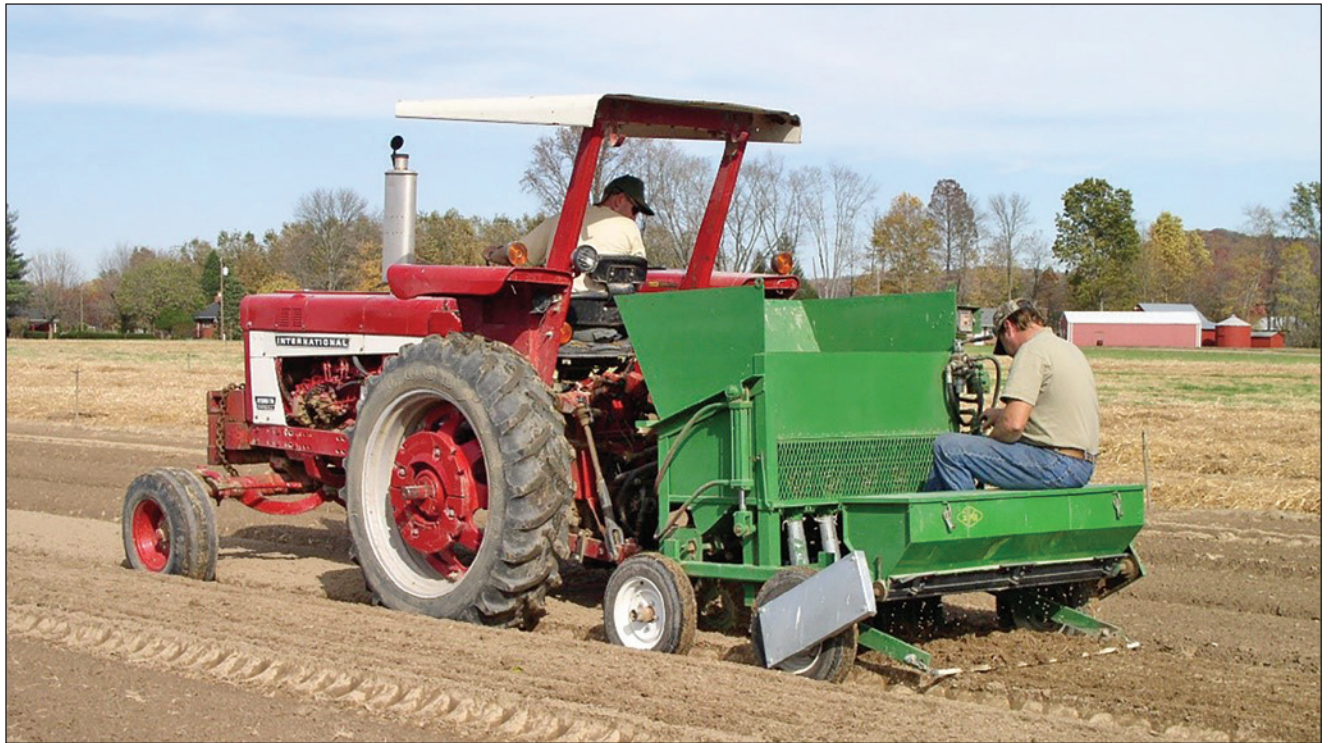
Figure 4a.4 —Operation of a large acorn seeder. This seeder was built at the Vallonia State Nursery in Indiana. A living mulch seed sower attached to the back of the acorn sower sows wheat, rye, or oats simultaneous to acorns. (Photo by Jeanie Redicker, Indiana Department of Natural Resources, 2013.)
