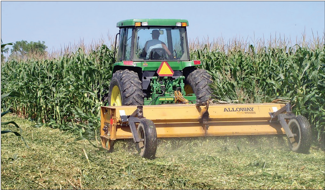
Figure 4a.1 —Flail mower used to cut cover crop prior to soil preparation. Mowing is followed by incorporation (disking), fumigation, and bed preparation. (Photo by Jeanie Redicker, Indiana Department of Natural Resources, 2013.)
