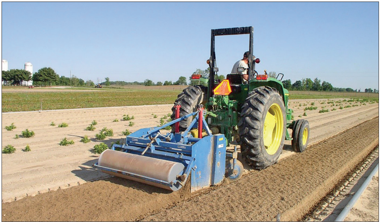
Figure 4a.2 —Bedformers have soil rototilling functions in addition to the formation of a specific bed width. (Photo by Jeanie Redicker, Indiana Department of Natural Resources, 2013.)
