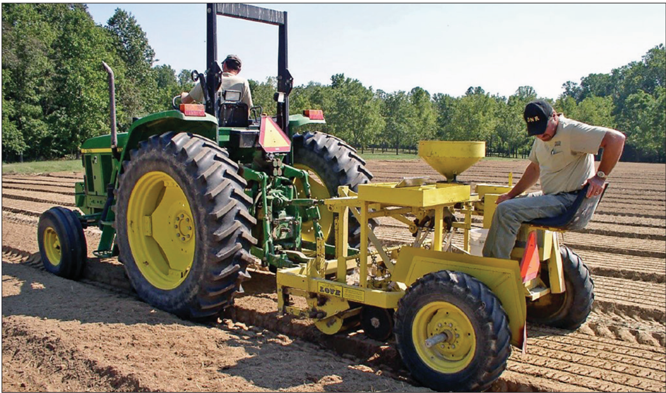
Figure 4a.3 —Operation of the Love seed drill, used for small-seeded hardwood sowing. (Photo by Jeanie Redicker, Indiana Department of Natural Resources, 2013.)
