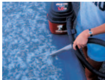
A 1-horsepower shop vacuum sucks the cotton and seeds through the window screen—coarser debris remains behind. Inside the vacuum, the cotton sticks to the cloth filter and the seeds collect in the bottom of the canister.
