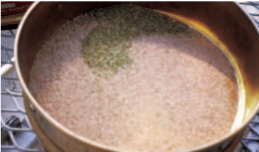
Figure 3. The mostly clean aspen seeds that collect in the passive shop vacuum are poured into a #18 round test sieve (top) where the coarse debris remains (middle) and the seeds pass through onto a #35 round test sieve (bottom). These sieves are the same as those used for soil sampling.
