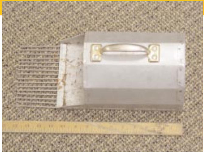
Figure 2. A custom-made metal harvester for collecting fruits.
