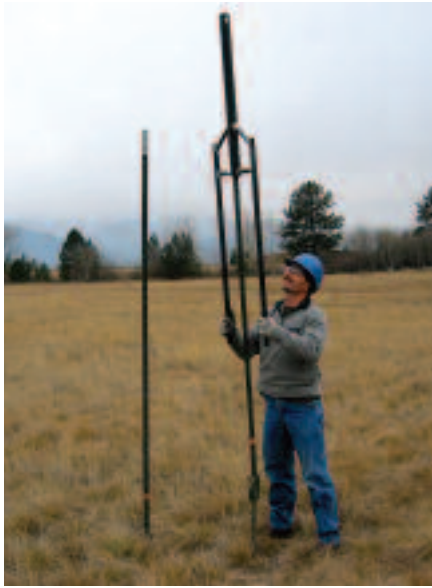
Figure 6. This fence-post driver designed by MTDC helps workers install 10 ft long (3 m) posts without using ladders.
