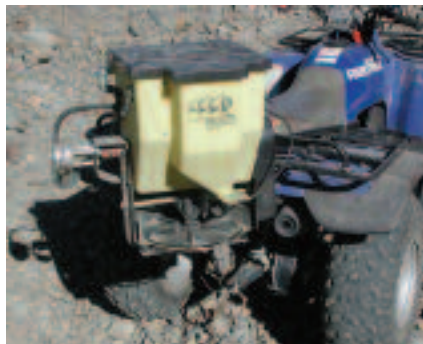
Figure 2. Truax Seed Slinger has separate hoppers for fluffy seed and for small flowable seed.
