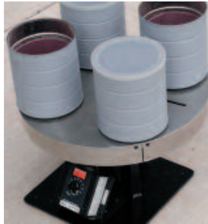
Figure 7. Seeds in the whitebark pine seed scarifier swirl across sandpaper that lines each of the four cans.
