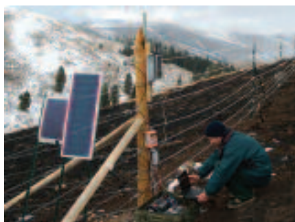
Figure 4. Six ft tall (1.8 m), high-tensile steel electric fences and polyrope electric fences were charged with a battery and solar panels.
