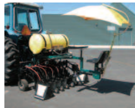
Figure 1. The MTDC shielded herbicide sprayer has adjustable spray hoods and a tiller steering system.
