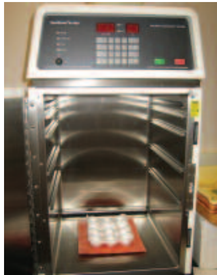
Figure 2. Indented carton of acorns on top of photographic paper on bottom of X-ray machine. Photo by Rosa C Goodman
